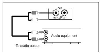
For playing the other equipment through this unit, connect between the audio output jacks on the other equipment and AUX jacks by using audio cords (not supplied).
